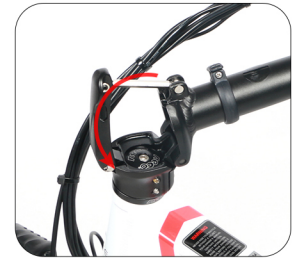
3 Put the riser pipe upright in the direction of the arrow and install it
