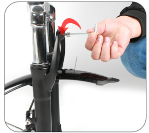
1 Loosen the front fork screws with a hexagonal screwdriver
