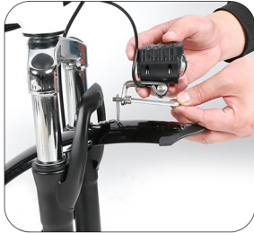
2 Put the headlights and the front fender into the screws and tighten them
