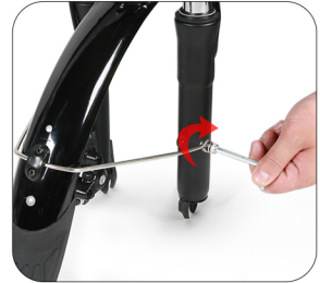
4 Tighten the brackets on both sides of the front fender
